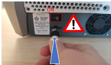
Figure 2: Be careful not to plug in the power supply when the switch is in the "On" position.
