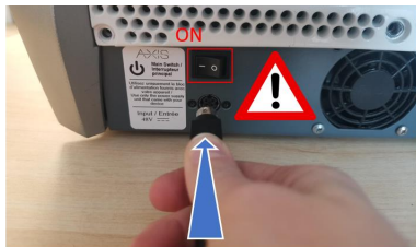
Figure 2: Be careful not to plug in the power supply when the switch is in the "On" position.
